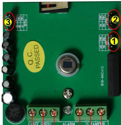
POWER GND Occupied Pulse Tamper Switch
